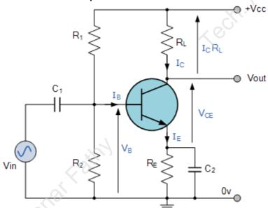
The single stage common emitter amplifier circuit shown above uses what is commonly called "Voltage Divider Biasing". This type of biasing arrangement uses two resistors as a potential divider network across the supply with their center point supplying the required Base bias voltage to the transistor. Voltage divider biasing is commonly used in the design of bipolar transistor amplifier circuits.
