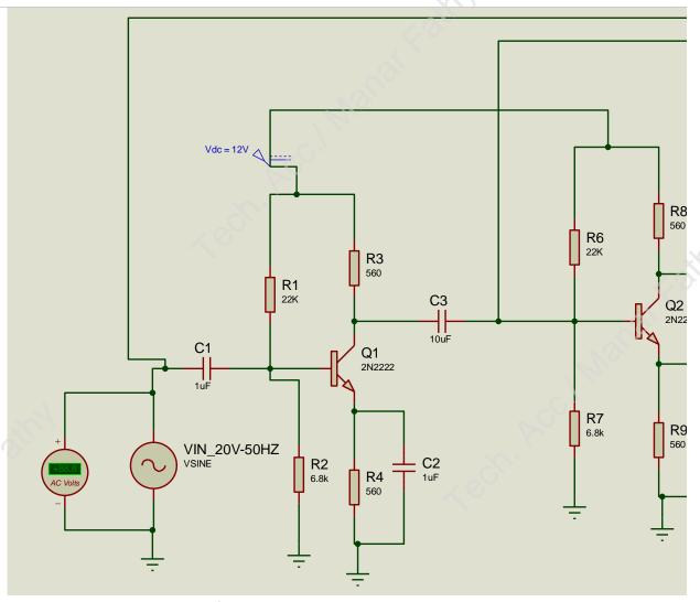
The multistage amplifier applications are it can be used to increase extremely weak signals to utilizable levels. The distortion can be reduced by changing the signal within stages. At present, any electronic device can process digital or radio electrical signals by including a multistage amplifier.
