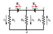
**Figure 7.5:** A multi loop circuit consisting of three branches: left-hand branch (*bad*), right hand branch (*bcd*), and central branch (*bd*). The circuit also consists of three loops: left hand loop (*badb*), right-hand loop (*bcdb*), and big loop (*badcb*).
