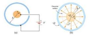
Figure 5.5: Spherical capacitor
