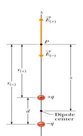
**Figure 2.5**: Electric field due to an electric dipole at a Point on its axis
