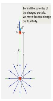
Figure 4.4: Potential due to point charge
