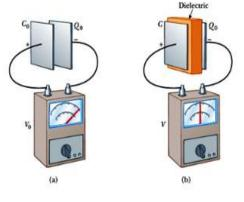
**Figure 5.6:** Capacitor a) without dielectric. b) with dielectric.
