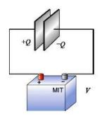
the terminals, and a decrease in the terminal voltage. Chemical **Figure 5.7:** Capacitor in a circuit. reactions are then triggered to transfer more charge from one terminal to the other to compensate for the loss of charge to the capacitor plates, and maintain the terminal voltage at its initial level. The battery could thus be thought of as a charge pump that brings a charge (*Q*) from one plate to the other.
