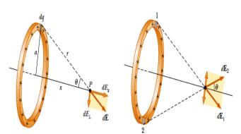
**Figure 2.7**: The electric field of a uniform charged ring along its central axis.
