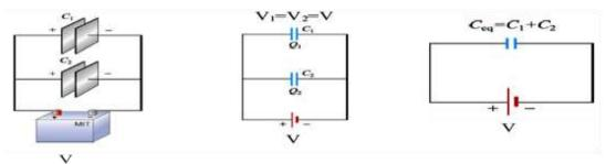
Figure 5.8: Parallel Connection of capacitor in a circuit.
