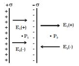
Figure 3.9: Two parallel infinite non-conducting sheets
