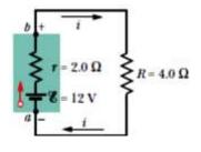
**Figure 7.6:** Points (*a*) and (*b*), which are at the terminals of a real battery, differ in potential.
