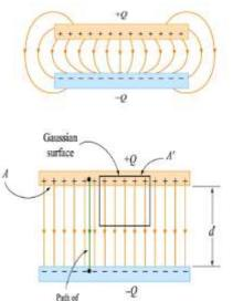
**Figure 5.3:** Parallel plates capacitor
