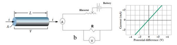
Figure 6.5: A potential difference (V) is applied between the ends of a wire of length (L) and cross section
