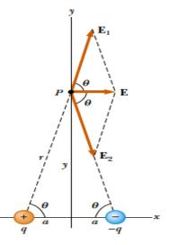
**Figure 2.6**: Electric field due to an electric dipole at a point on the equatorial line.
