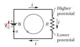
**Figure 7.4:** A single-loop circuit in which a resistance (*R*) is connected across an ideal battery (*B*) with emf ( $\varepsilon$ ). The resulting current (*i*) is the same throughout the circuit.
