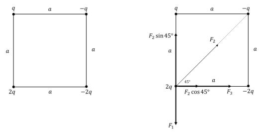
the repulsion force between charge (2q) and (q) at the corner of square along y - axis
