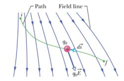
**Figure 4.2:** Moveing of test charge  $(q_0)$  in an electric field.
