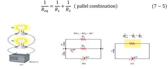
**Figure 7.3:** (a) A parallel connection of two lightbulbs with resistances  $(R_1)$  and  $(R_2)$ . (b) Circuit diagram for the two-resistor circuit. The potential differences across  $(R_1)$  and  $(R_2)$  are the same. (c) The equivalent resistance of the combination is given by the reciprocal relationship  $(1/R_{eq} = 1/R_1 + 1/R_2)$ .
