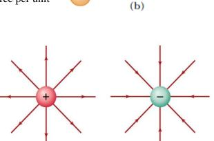
**Figure 2.3**: The electric field lines for a positive point charge, the lines are directed radially outward and are directed radially inward for a negative point charge
