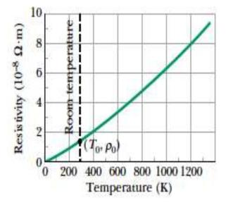
**Figure 6.6:** The resistivity of copper as a function of temperature. The dot on the curve marks a convenient reference point at temperature ( $T_o = 293 \text{ K}$ ) and resistivity ( $\rho_o = 1.69 \times 10^{-8} \Omega \cdot m$ ).
